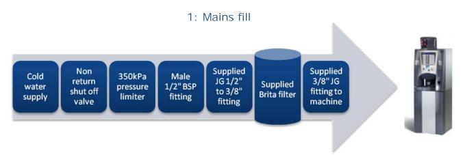
The mains option requires a cold drinking water supply within 2m. This should be from an accessible, non return, water shut off tap fitted with a 1/2" BSP male fitting. 2m of John Guest water line is supplied which is cut as needed for the supply to the machine.
