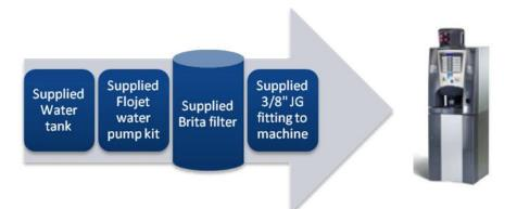
The tank option needs only electrical power; tank and plumbing fittings are fitted ready for use.
